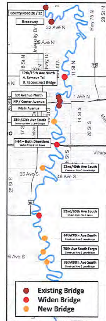
POTENTIAL RED RIVER BRIDGE CROSSINGS ALTERNATIVES
